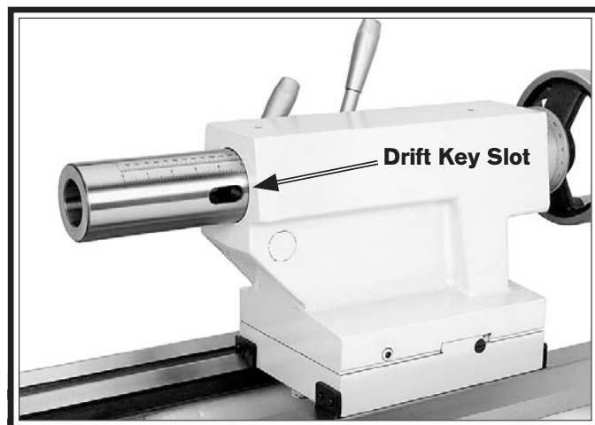
Figure 51. Drift key slot in the side of the quill.
