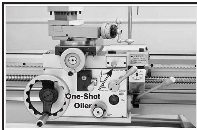
Figure 105. Location of one-shot oiler on the apron.
