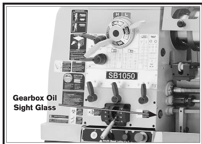
Figure 101. Location of quick-change gearbox oil sight glass.
