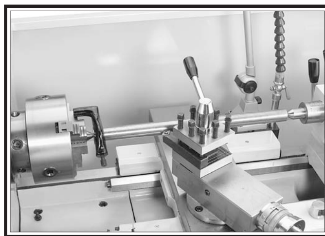
Figure 54. Example photo of a workpiece mounted between the centers.
