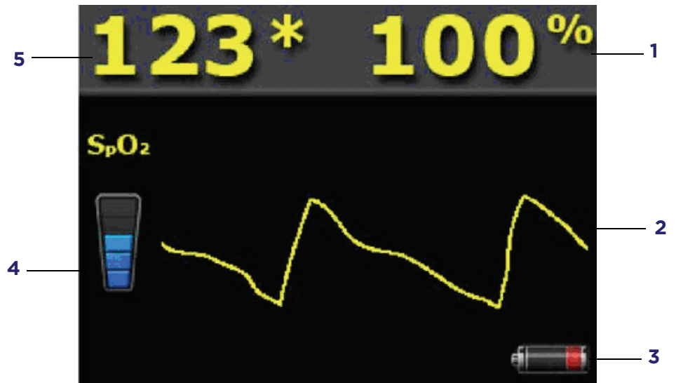
Figure 4-7 Typical SpO 2 display on 96281-C (shows a low battery state)
