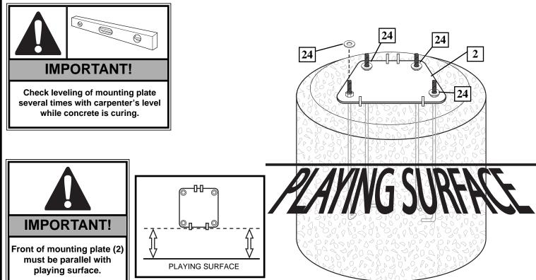
IMPORTANT!: WAIT A MINIMUM OF 72 HOURS BEFORE GOING ON TO NEXT STEP. CONCRETE MUST CURE. ALLOW ADDITIONAL TIME FOR COLD, WET OR HUMID WEATHER.
