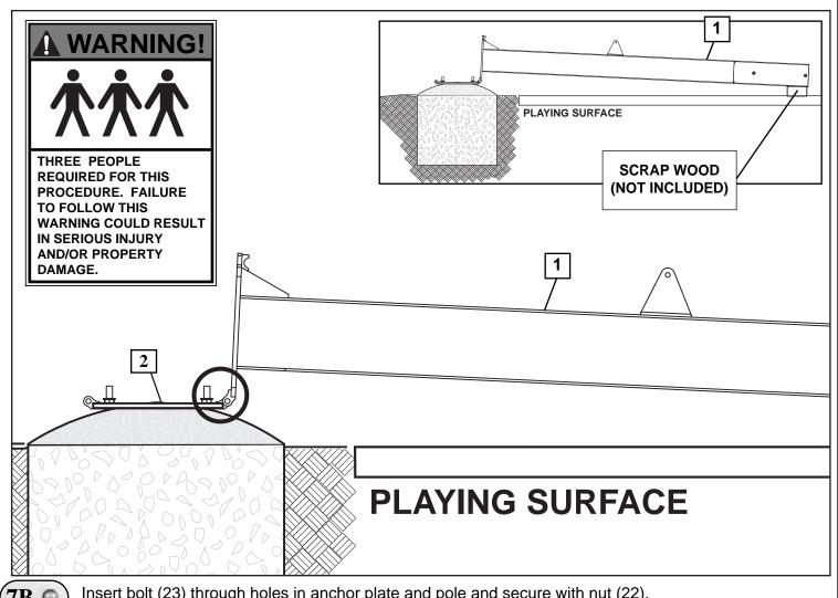
Insert bolt (23) through holes in anchor plate and pole and secure with nut (22). 7B.♀
