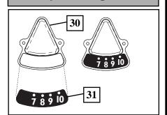
Attach height indicators to lower yoke in area shown by turning screws (B. © (29) into place with a phillips-head screwdriver. Apply name plate sticker (15) to lower yoke as shown.
