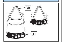
B. Attach height indicators to lower yoke in area shown by turning screws (29) into place with a Phillips head screwdriver.
