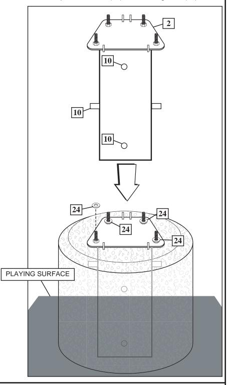
IMPORTANT!: WAIT A <u>MINIMUM</u> OF 72 HOURS BEFORE GOING ON TO NEXT STEP. CONCRETE <u>MUST</u> CURE. ALLOW ADDITIONAL TIME FOR COLD, WET OR HUMID WEATHER.
