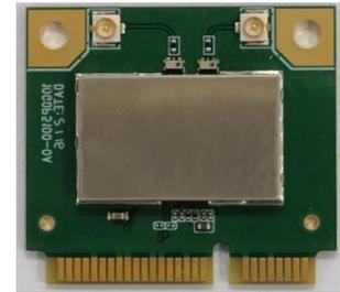
SparkLAN **WPET-239ACN(BT)** is a highly integrated single-chip Wireless LAN (WLAN), Bluetooth module which supports 2 streams 802.11ac solutions with multi-user MIMO (Multiple-Input, Multiple-Output) wireless LAN (WLAN) and integrated Bluetooth 5.0. It is integrated 2Tx2R WLAN MAC, baseband, and dual band RF in a single chip module. **WPET-239ACN(BT)** provides a cost effective solution for M2M (machine to machine) connectivity product/device by PCIe.
