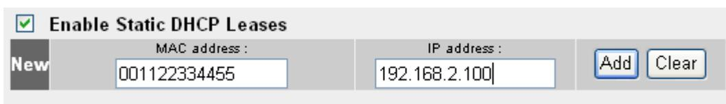
The screenshot shows a configuration window for static DHCP leases. At the top, there is a checkbox labeled 'Enable Static DHCP Leases' which is checked. Below this, there is a 'New' button on the left. To its right are two input fields: 'MAC address' containing '001122334455' and 'IP address' containing '192.168.2.100'. To the right of these fields are two buttons: 'Add' and 'Clear'.
