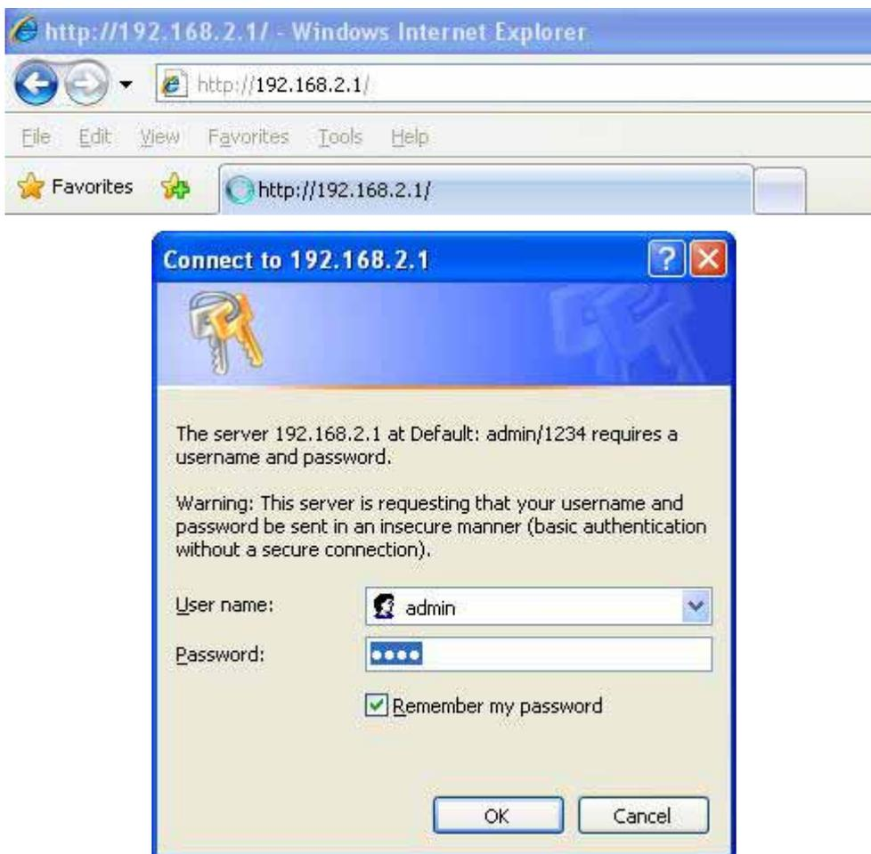
In order to configure the SpeedPlus Wireless-G AP/Router, you must input the password into the **Password** box and leave blank on the **User Name** box. The default User name is “**admin**” and password is “**1234**”.
