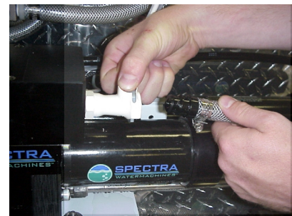
Connecting the brine discharge service hose
