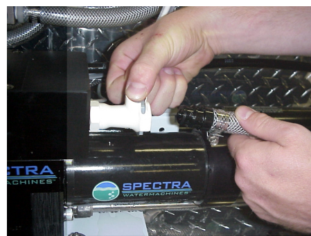
Connecting brine discharge hose
