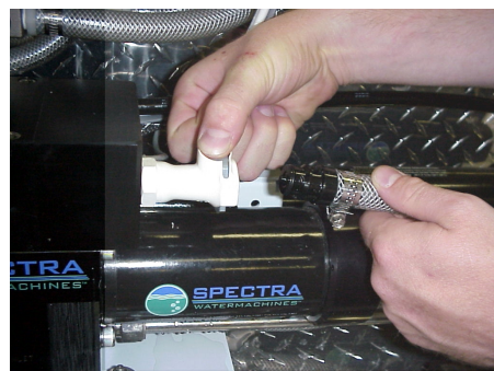
Connecting brine discharge hose
