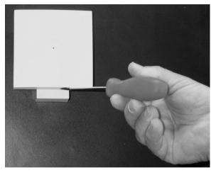
If you need to remove the Repeater please separate it from the wall holder with a gentle push of a screwdriver.
