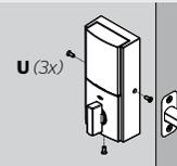
Note: The interior cover and screws must be removed for battery pack access.
