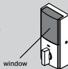
If you wish to unlock the window, you can slide it up for more convenient access to the programming buttons while the cover is installed.
