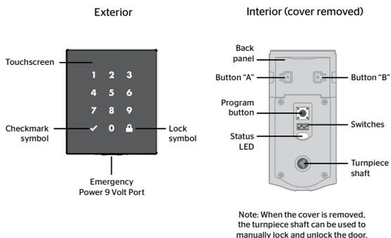
Note: When the cover is removed, the turnpiece shaft can be used to manually lock and unlock the door.
