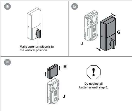
**B** Install interior assembly onto mounting plate.
