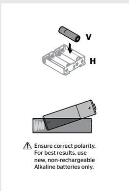
**B** Make sure the door is open, and insert the battery pack.
