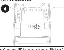
**4.** Charging LED indicates charging. Blinking for charging and solid ON when fully charged.
