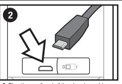
2. Plug the small end of the charging cable into the charging port.
