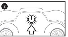
**2.** Hold the controller near your truck, press the power button and wait until power light stops flashing.
