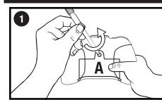
**1.** Open the battery door with a screwdriver (A). If used batteries are present, remove these batteries from the unit by pulling up on one end of each battery. DO NOT remove or install batteries using sharp or metal tools.
