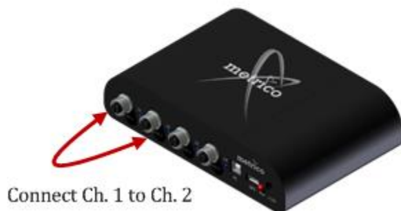
Figure 9-1 – Hardware Configuration for Voice Quality Test Calibration on a Nomad ME unit
