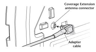
**5. Connect RG6 to Coverage Extension Antenna** Connect the other end of the RG6 cable to the
