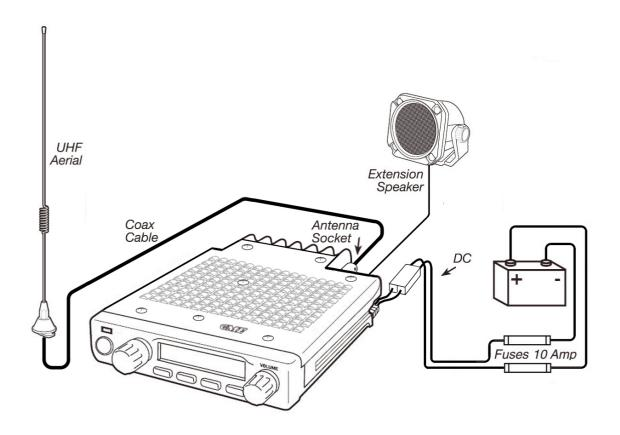
Two in-line 10 Amp fuses are supplied. These fuses are to be connected as close to the battery as possible. The radio's positive (red) lead should be connected via a 10 Amp fuse directly to the battery's positive terminal. Connect the radio's negative (black) lead via a 10 Amp fuse directly to the battery's negative terminal.
