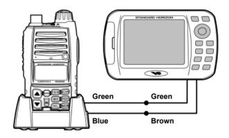
To connect the GPS receiver, connect the wires between the **CD-33** and the GPS. Insure that the wires are properly shielded from water. See the figure at the right for example of connection to STANDARD HORIZON GPS CHART PLOTTER.
