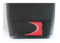
Place the battery in its compartment
