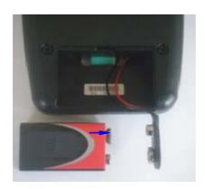
Connect the 9V battery to the connector respecting the polarity.
