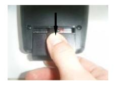
Remove the battery compartment cover by lightly pressing with the end of your finger.
