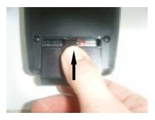
To close the battery compartment cover – follow the slides – lightly press the cover into place with the end of your finger
