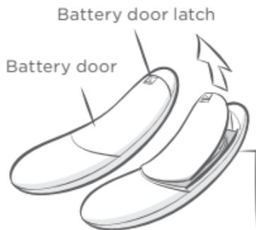
Unclip latch and rotate open
