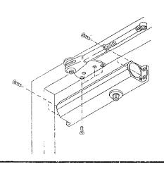
4. OPEN DOOR TO THE DESIRED HOLD OPEN ANGLE AND FIRMLY FASTEN LOCKING BOLT WITH A SPANNER.
