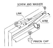
NOTE: ADJUST LENGTH OF ADJUSTABLE LINK TO KEEP CLEAR BETWEEN ARM AND DOOR SURFACE.
