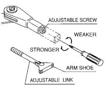
3. POSITION STANDARD ARM SHOE ON FRAME AND FASTEN WITH TWO SCREWS.
