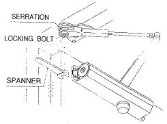
NOTE: DAMAGE TO THE HOLD OPEN DEVICE MAY OCCUR IF THE LOCKING BOLT IS NOT FIRMLY TIGHTENED.
