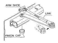
NOTE: ADJUST LENGTH OF ADJUSTABLE LINK TO OBTAIN A 90° ANGLE TO DOOR.
