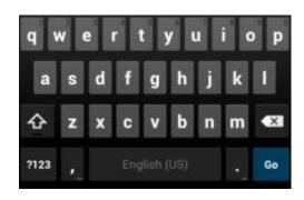
То delete character То enter an , and then tap that upper-case letter letter. To enter a digit , and then tap that Tap digit. To enter a symbol , and then tap that symbol. Press the space key twice Quickly enter successively. space To toggle input Hold down to to bring up methods the keyboard.
