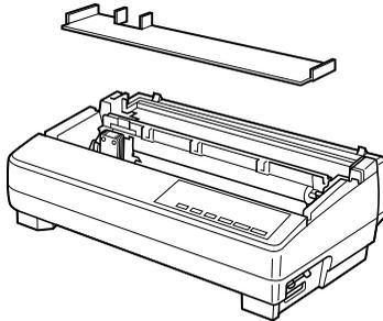
In addition, remove the cardboard from the back of the paper guide.
