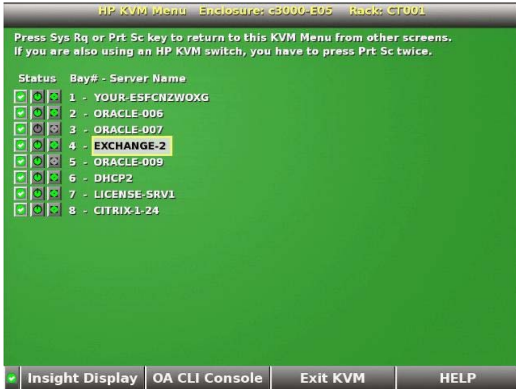
Figure 7. Optional c3000 KVM Module – KVM menu screen
