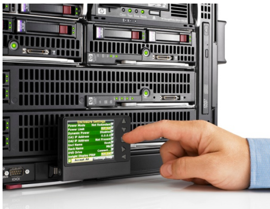
Figure 4. Insight Display on the c3000 enclosure
