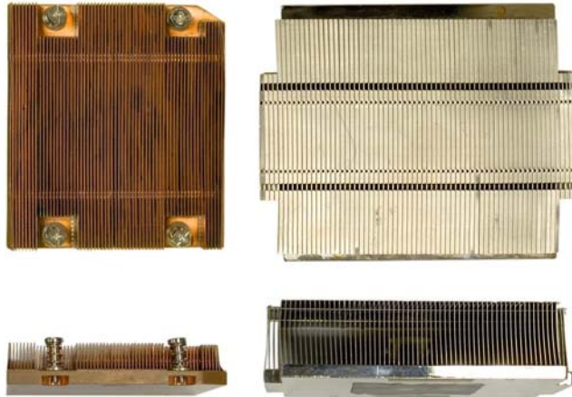
Figure 18. Processor heat sink using fully ducted design (left) and a traditional heat sink in a 1U rack-mount server (right)
