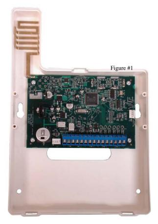
You can double the maximum wire length if you double the conductors and connect them in parallel. Mount the TLR as close to the power supply as possible.
