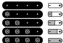
3. All four LEDs will flash ON and OFF evenly when the Controller is not paired.
