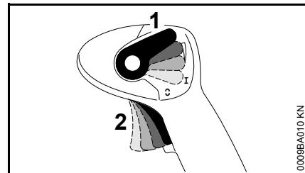
The throttle trigger (2) can be locked in any position by operating the setting lever (1).
