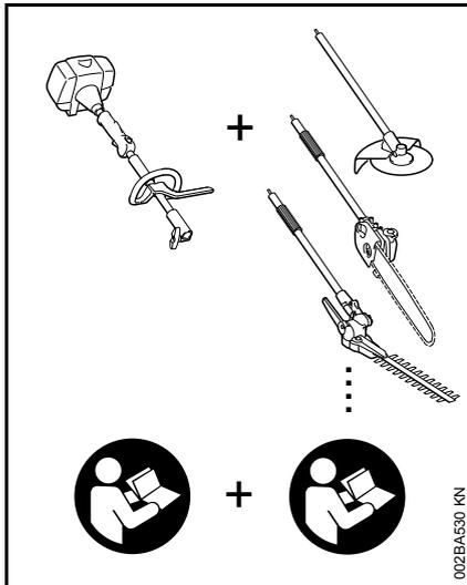
In the STIHL KombiSystem a number of different KombiEngines and KombiTools can be combined to produce a power tool. In this instruction manual the functional unit formed by the KombiEngine **and** KombiTools is referred to as the power tool.
