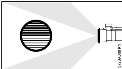
Splits the spray jet in two – allows two closely planted rows to be treated simultaneously.
