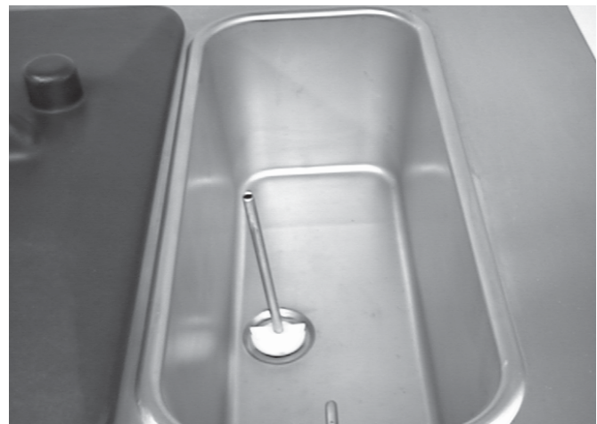
Figure 27. Install Mix Inlet Regulators
