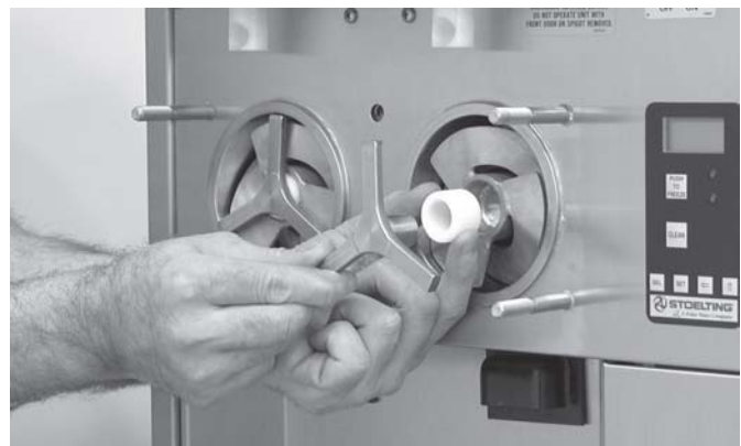
Figure 23. Removing Auger Supports
