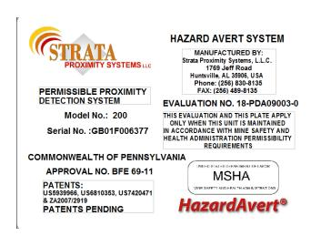
The Strata label defines the model and serial number of the Underground Proximity Generator. The MSHA label provides the MSHA approval number and specific MSHA certification.
