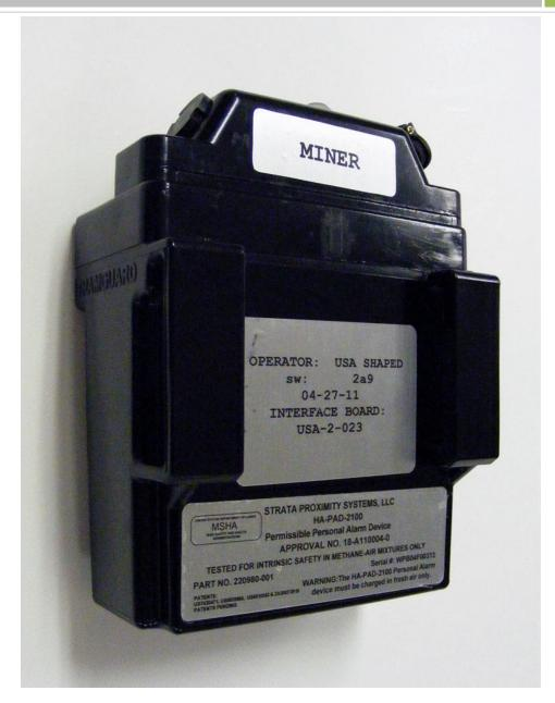
The Strata label defined the Software (sw) version and Interface model number used inside the PAD. The MSHA label provides the MSHA approval number, specific MSHA certification, serial number and operational warning for fresh air charging only.
