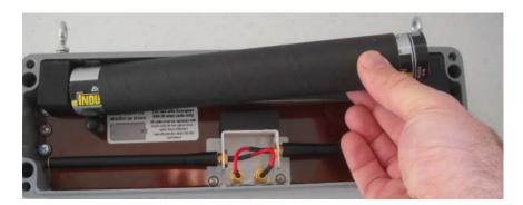
Use the supplied non-conductive tool to guide the positive end of the battery tube into position.
