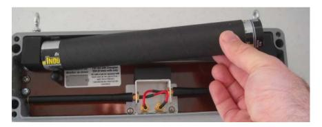
Remove the four (4) D cell batteries from the tube, if present, and dispose of properly.
