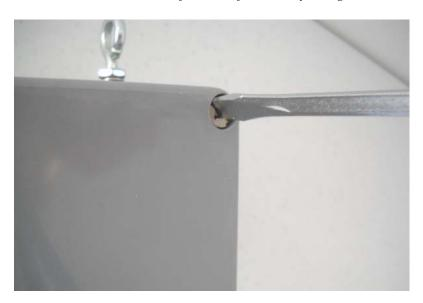
A small no conductive tool is within the C201 enclosure to ease insertion of batteries.
