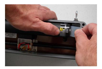
Remove the guide tool from between the battery and contact. This powers on the C201. If batteries are being installed in a storage or staging area, leave the guide tool in place so that the C201 is not powered on. The C201 is not to be powered on until it is at its installation location.
