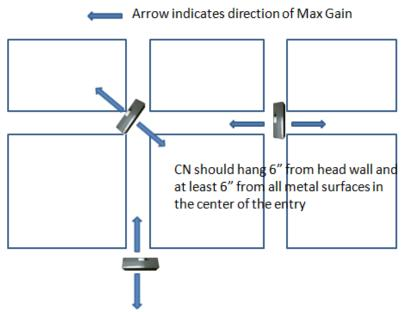
Signal strength example looking from above down onto the mine
