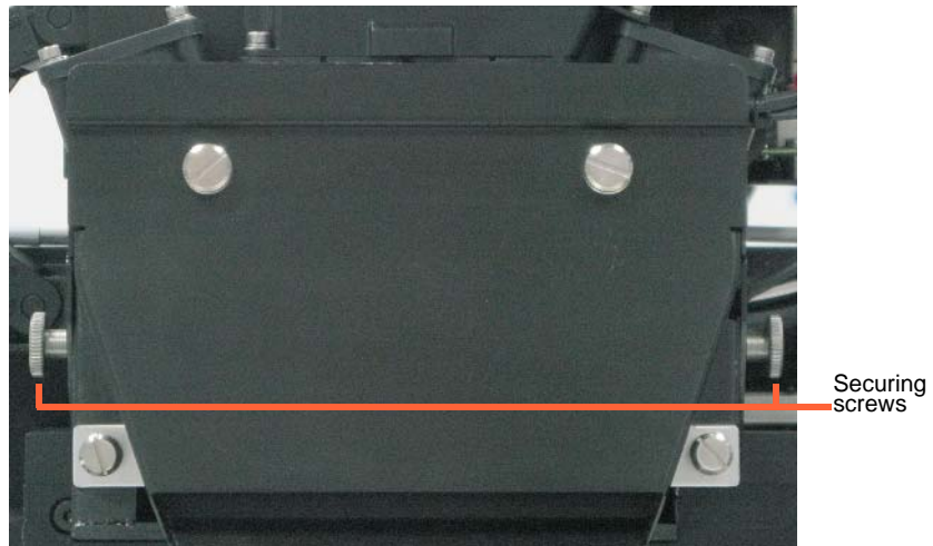
Figure 7-40: UV-lamp-assembly securing screws
