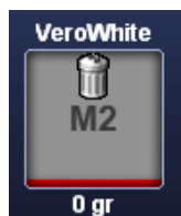
Figure 7-6: Empty cartridge indicator
