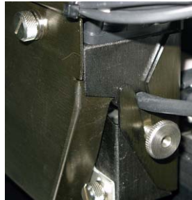
Figure 7-79: UV-lamp cable after replacing the assembly
