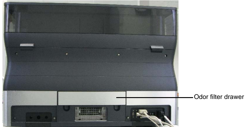
Figure 7-69: Rear of the Alaris30 printer
