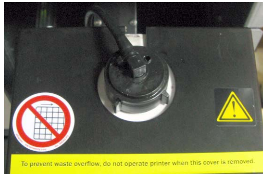
Figure 7-85: Fireproof cover installed over the waste container
