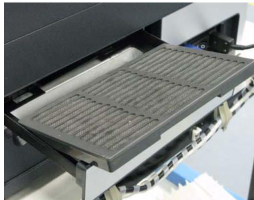
Figure 7-70: Odor filter in drawer
