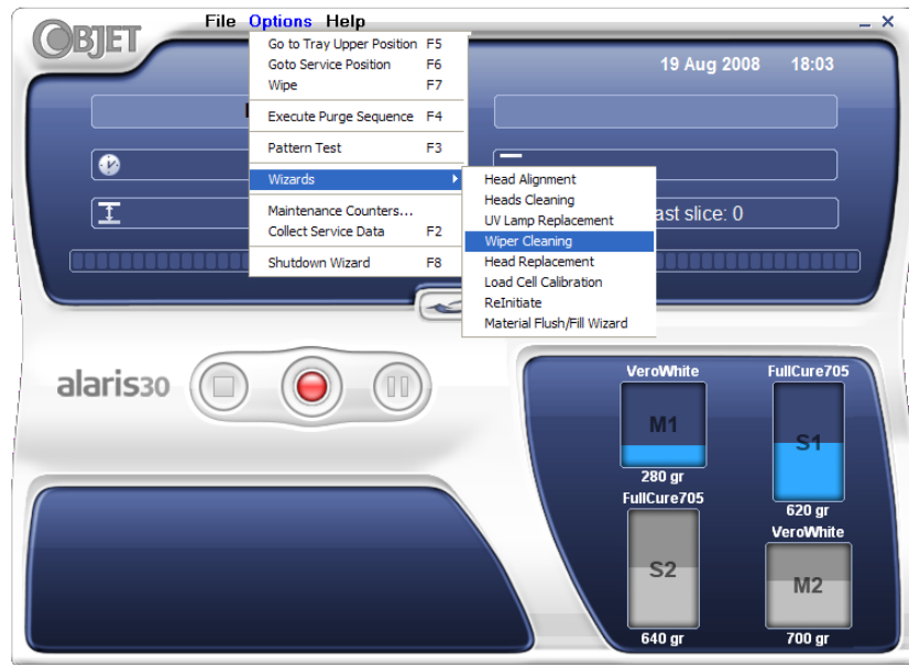
Figure 7-33: Starting the Wiper Cleaning wizard
