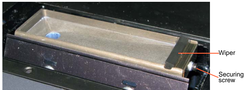
Figure 7-36: Wiper and excess-material drain
