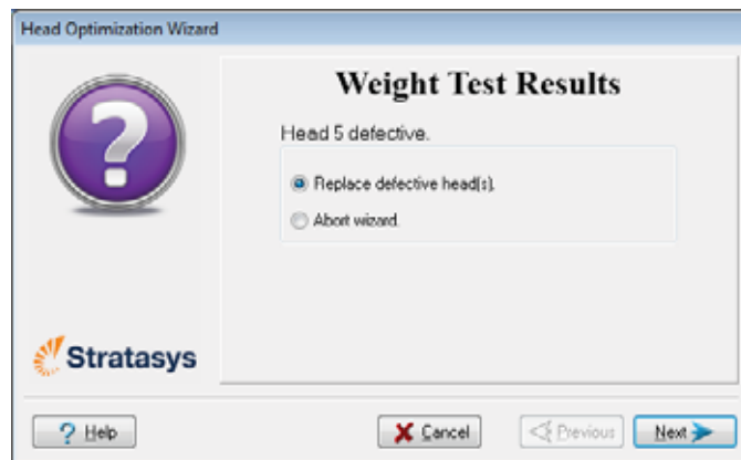
Figure 6-60: Defective print heads found
