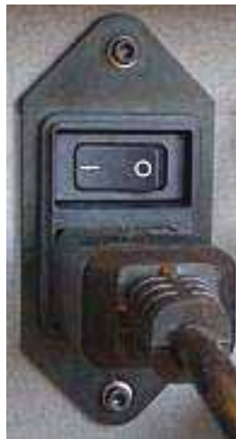
Figure 6-2: Main power switch and cable
