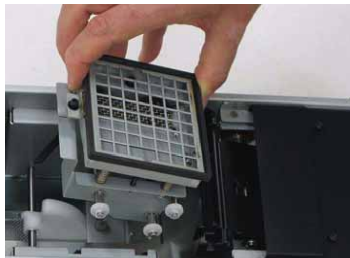
Figure 6-25: Purge unit waste collector
