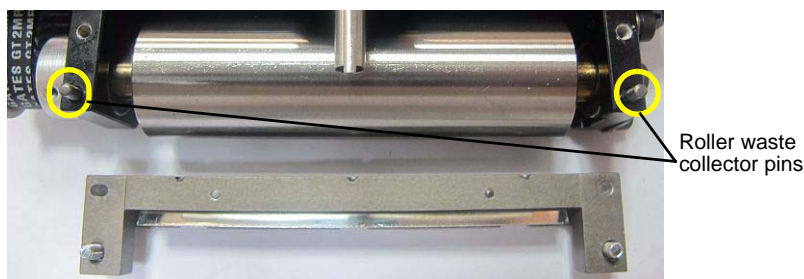
Figure 6-30: Roller waste collector pins
