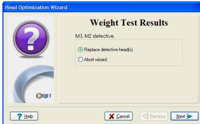
Figure 7-56: Defective print heads found
