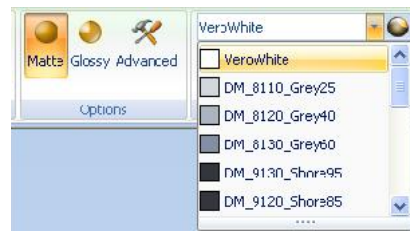
Figure 5-28: Menu for assigning materials to objects
