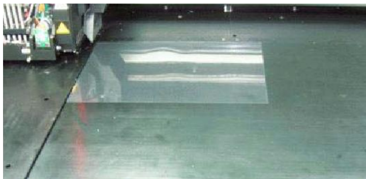
Figure 6-39: Positioning the transparency on the build tray
