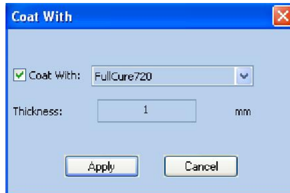
Figure 5-29: Coating material selected
