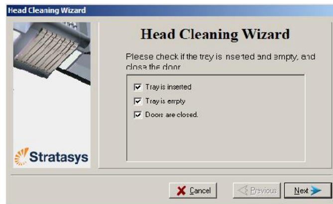
Figure 6-17: Head cleaning procedure—wizard screen
