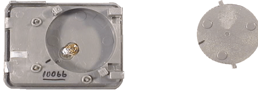
Figure 3: Installing the battery in the PID
