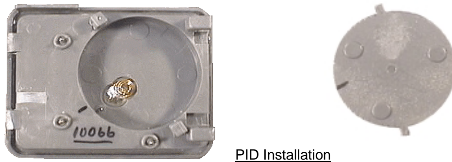
Figure 3: Installing the battery in the PID
