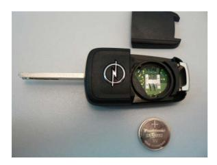
Replace the new battery +-side facing up. Avoid touching the new batteries with fingers, skin oils may cause battery deterioration. Do not touch the PCB or the battery clip.
