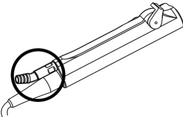
4. Connect suction tubing (for all suction-capable devices).
