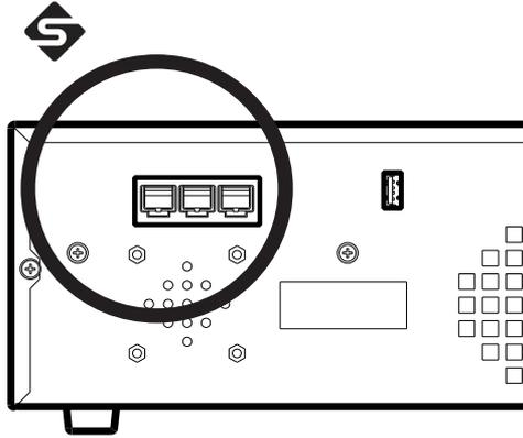
1. Connect the Crossfire™ console to the iSWITCH™ console using one of the Firewire connection ports on each console.
