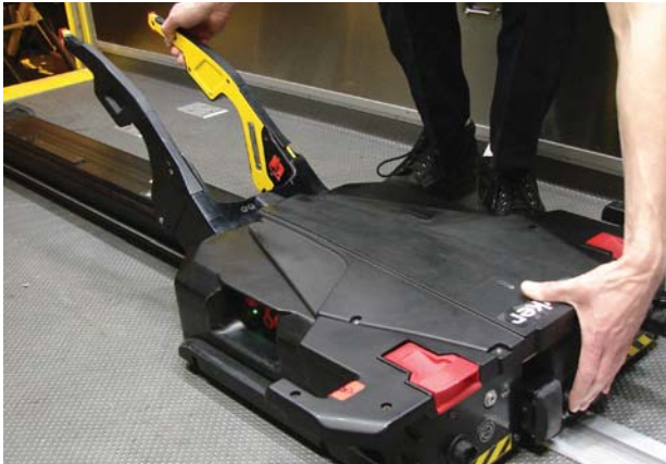
Figure 33: Press Manual Trolley Release Button
