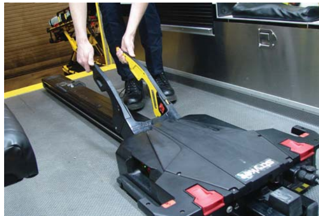
Figure 34: Pull Trolley Out
