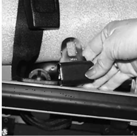
Figure 52.3: Securing the Safety Restraints on a Cot
