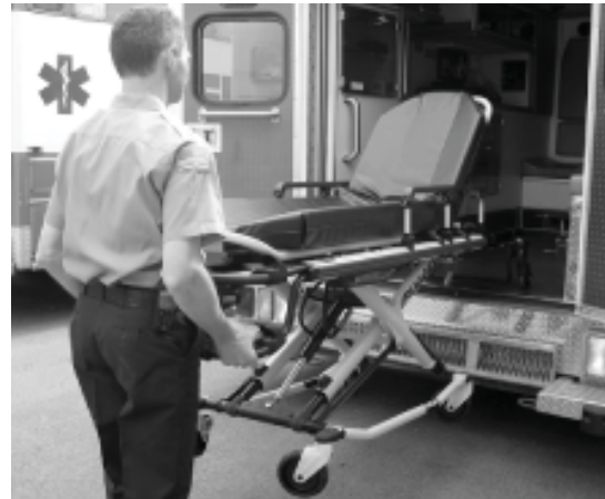
Figure 34: Pull the Manual Back-up Release Handle and Roll the Cot out of the Vehicle
