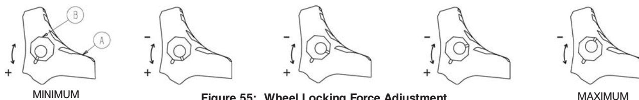
Figure 55: Wheel Locking Force Adjustment
