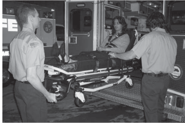
Figure 30: 2 Operators Unloading the Cot
