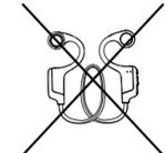
Do not twist or bend the rear hanger excessively Avoid damage to internal light guide elements
