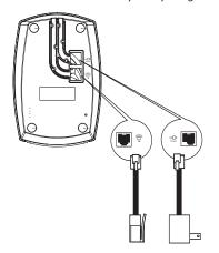
(2) Plug the other end of the line cord and power cable into the telephone wall socket and electrical power outlet. The line adapter may not be attached to the line cord. If this is the case, please connect the line cord to the line adapter before plugging it into the electrical outlet.
