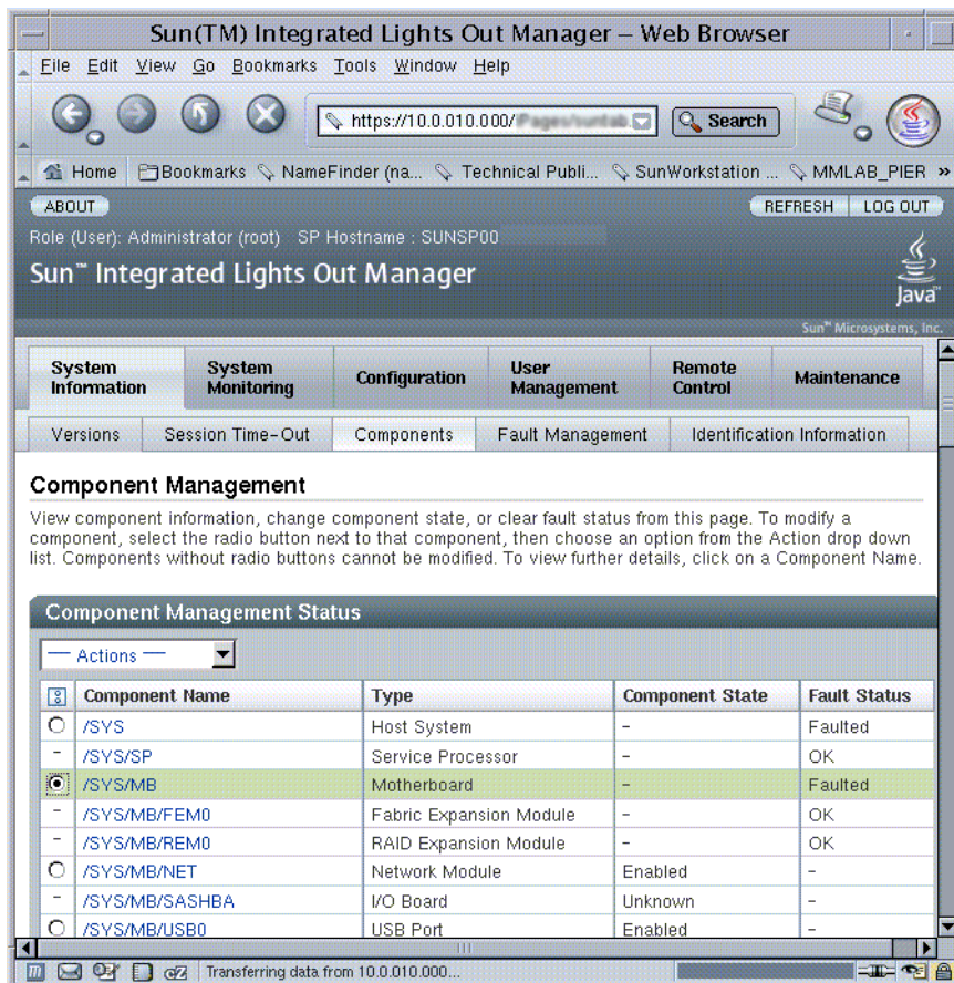
FIGURE 2-19 Enabling Components With the ILOM Web Interface
