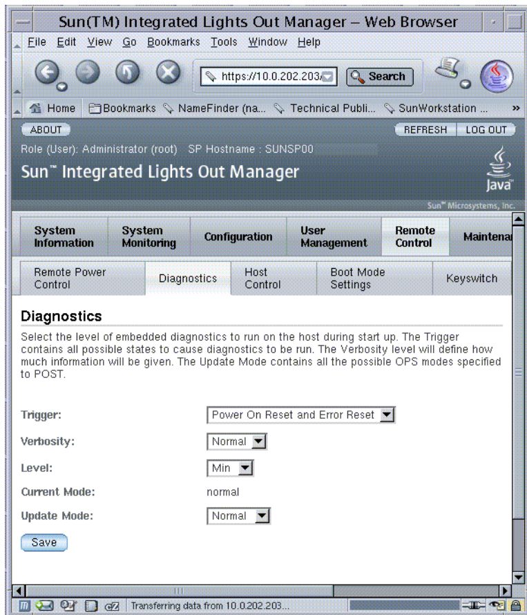
FIGURE 2-17 Setting POST Parameters With the ILOM Web Interface
