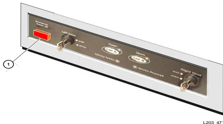
FIGURE 4-10 Emergency Robotic Stop Switch
