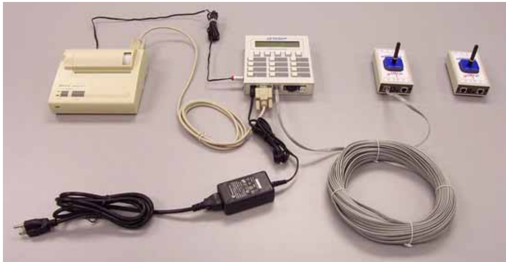
Figure 2-2. Typical wireless system connection with control module
