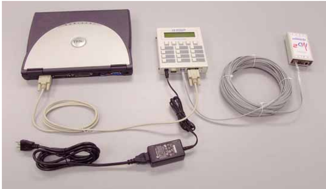
Figure 4-6. Typical serial port connection
