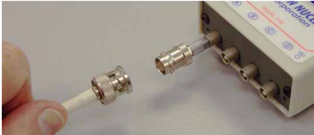
Figure 1-5. Using the BNC to LEMO adaptor
