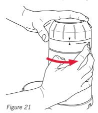
**Note:** The top burr can only be removed when the graphic arrow on the grind adjustment collar is aligned with the arrow on the motor base.
