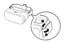
**2.**Buckle the hook to the top of front frame of VR, and pull up until it is firmly locked.
