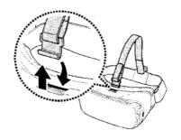
**3.** Slide the end of the headband through the ring in the main strap, and fix with Velcro firmly.
