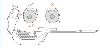
This device can load a 80mm thermal receipt or label paper roll, and black label is also optional.
