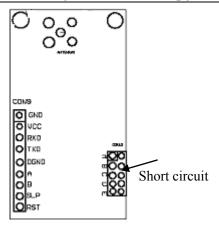
There is one group of 5-bit short-circuit wire (JP2) on the bottom right corner of SRWF-1022, defined as A、B、C、D、E respectively . A、B、C, D are used for channel selecting, but E is for parity format:
