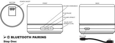
Turn the speaker on using the on/off switch located on the bottom of the device.
